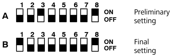
Fig. 51 Condensate drain timer (petrol units; Bürkert)
