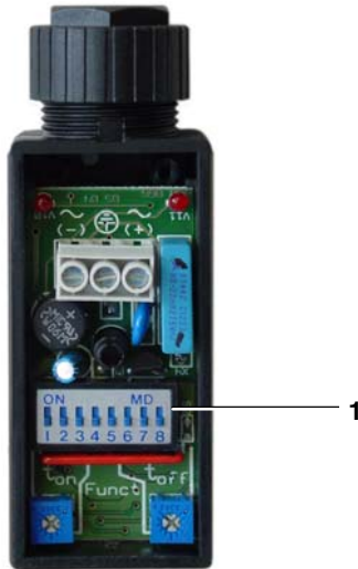
Fig. 51 Condensate drain timer (petrol units; Bürkert)
